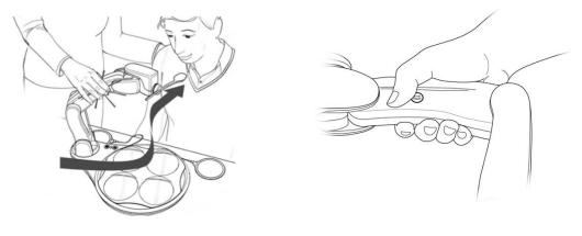
When the Teach Icon is covered, power will disengage from some motors and the Arm will allow movement. The last two sections of the Arm will remain engaged and will keep the Spoon level when moving within the workspace.
